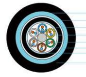
Double-side plastic coated steel tape Flooding jelly compound PE inner sheath Phosphating steel wire Fiber and filling jelly compound Flooding jelly compound Plastic coated aluminum strip PE Outer sheath
